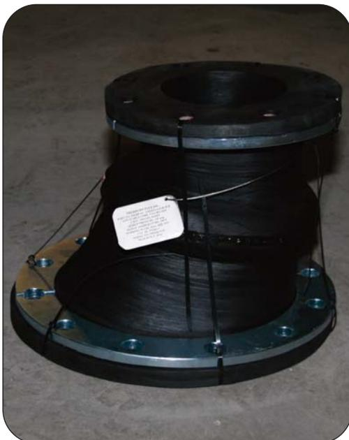
Thorburn's 42HPOX are custom rubber flexible pipes designed to replace rigid piping and absorb axial, lateral and angular movement caused by ground settling of storage tanks. Thorburn's 42HPOX can be manufactured with built in offsets, non parallel flanges with tangents to connect to existing storage tanks where angular and lateral offsets have occurred. Thorburn's 42HPOX can also be designed with multiple filled arches to provide smooth flow and prevent sediment build up in the arches.
