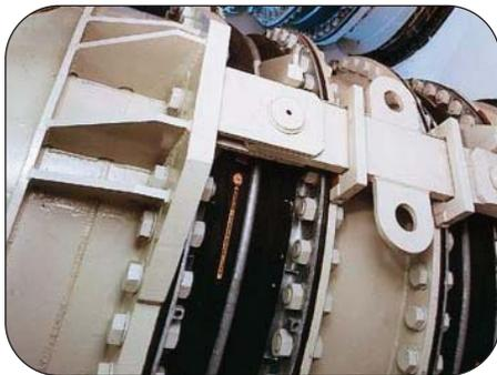
Thorburn's Rubber Hinge Expansion Joints are typically used in sets of two or three, to absorb pipe movement in one or more directions in a single plane piping system. Each individual joint in the system is restricted to pure angular rotation by its hinges.
