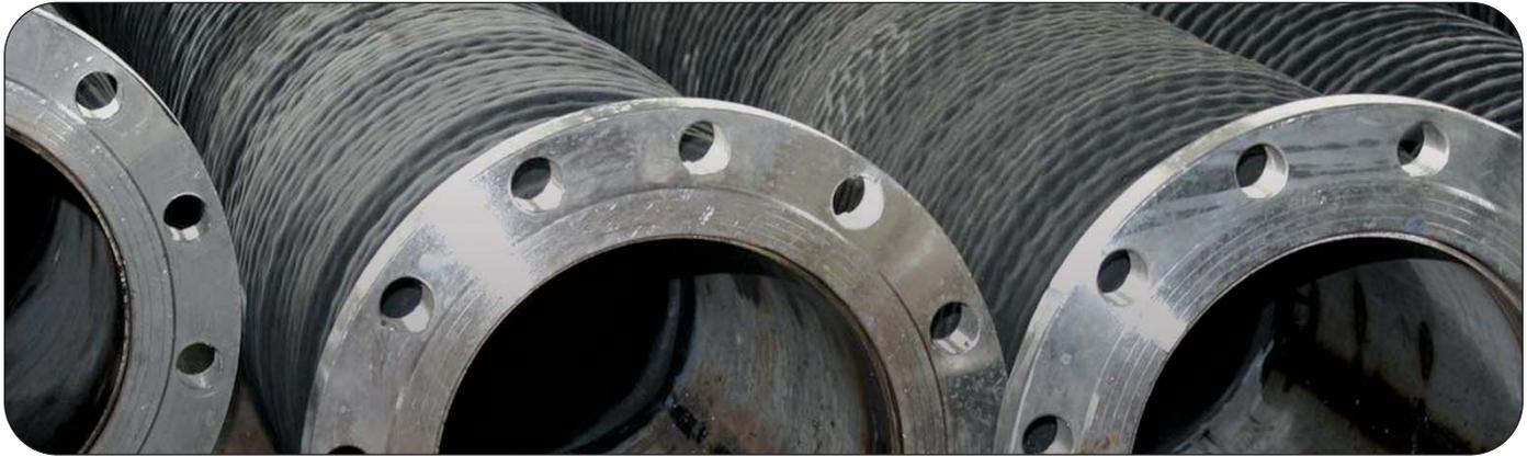
Thorburn 60TMH™ Flexpipe is a custom designed rubber piping system that replaces metal, rigid or flexible pipe and is used in lines requiring resistance to electrolysis, corrosion, abrasion and water hammering. 60TMH™ Flexpipe is specifically engineered for piping systems that require isolation and absorption of severe noise, vibration, misalignment, lateral deflection and flexing caused by thermal and mechanical movement.
